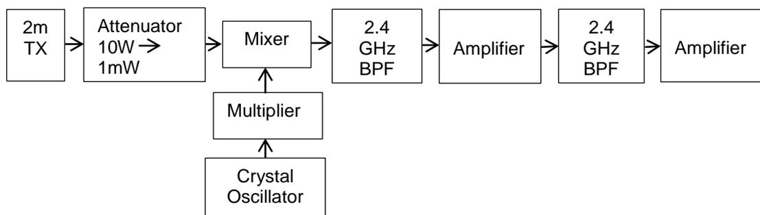
Figure 5: 2.4 GHz up converter block diagram.
