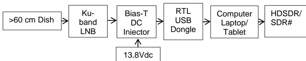
Figure 15: Possible Es'hail-2 receiver chain block diagram.
