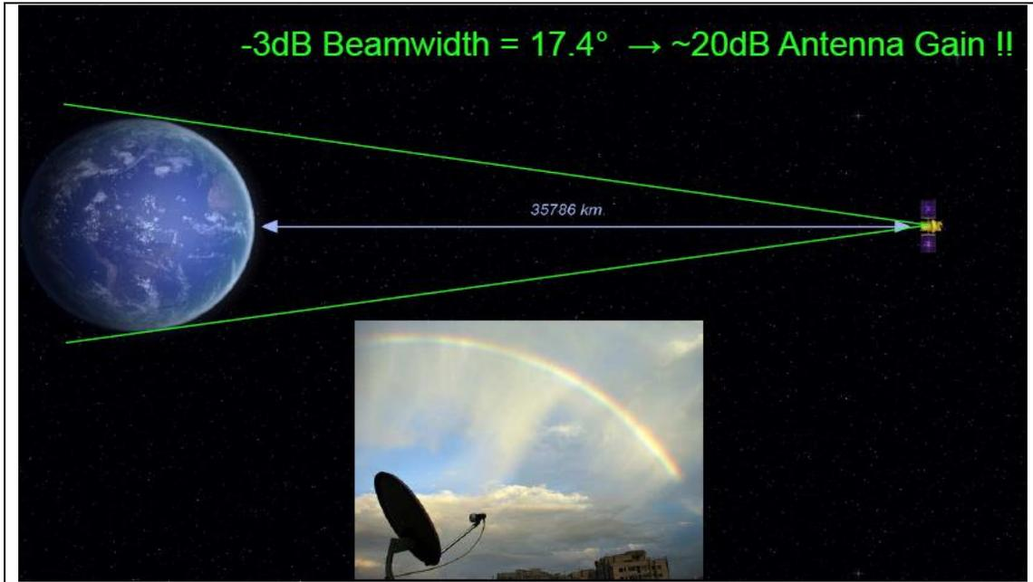
Figure 1: Angle of view from a geostationary satellite.
