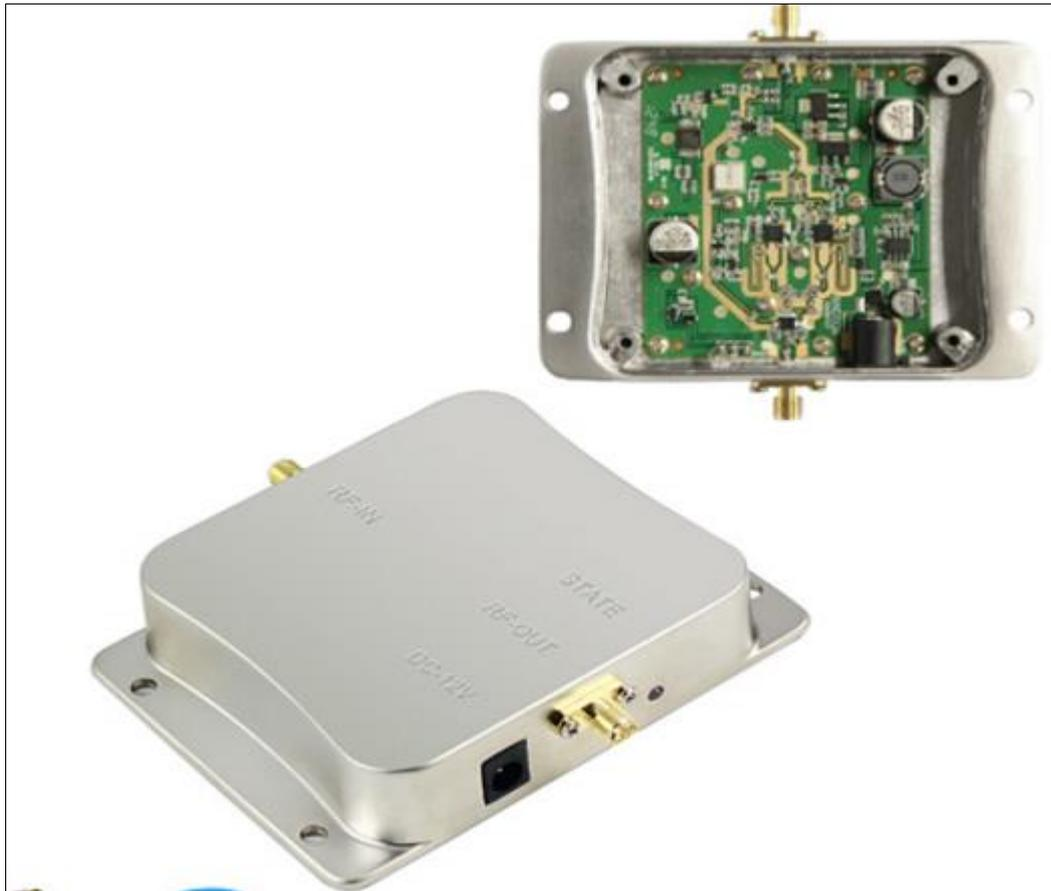
Figure 9: Packaged, 5 Watt, 2.4 GHz amplifier available from China.
