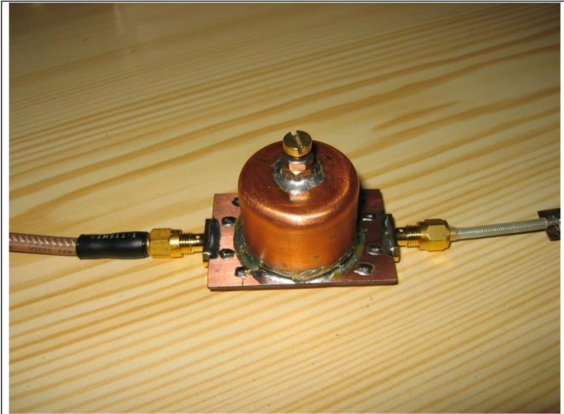
Figure 7: Example of a copper pipe cap bandpass filter.
