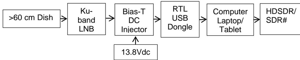
Figure 1: Possible Es'hail-2 ground station receiver chain.
