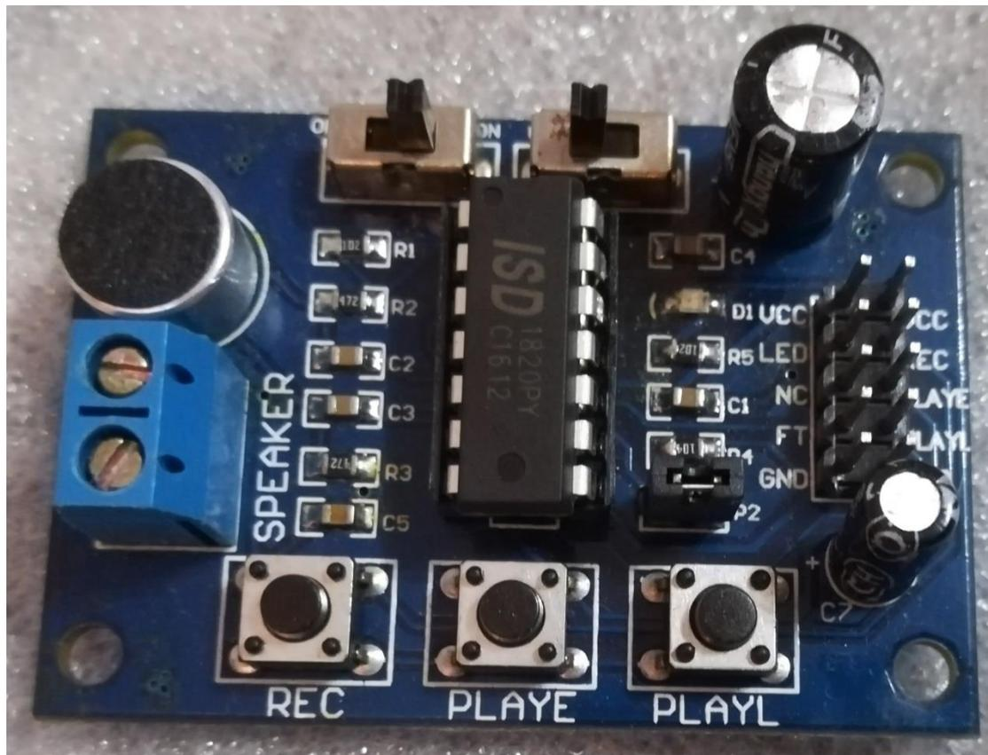
Figure 5: Electrothing voice storage module.
